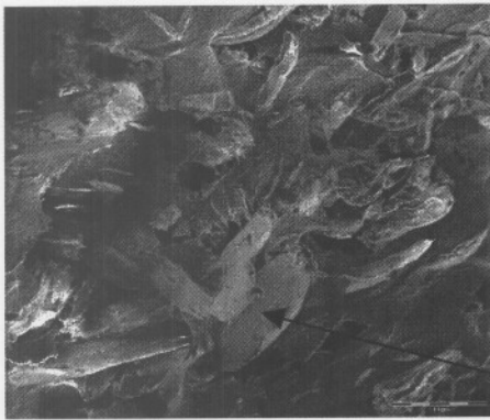
Figure 3-6: Microscopic view of drug particles inside a cross-cut Chit/EXPL bead.
