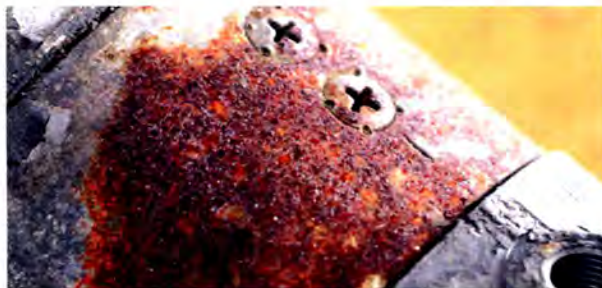
Figure 1.1: Iron oxide (rust)
