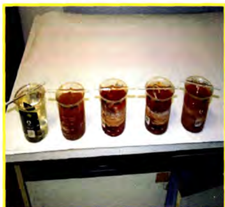
Figure 3.2: Experimental setup for the gravimetric procedure showing the metal sheets immersed in the solution with and without the inhibitor.
