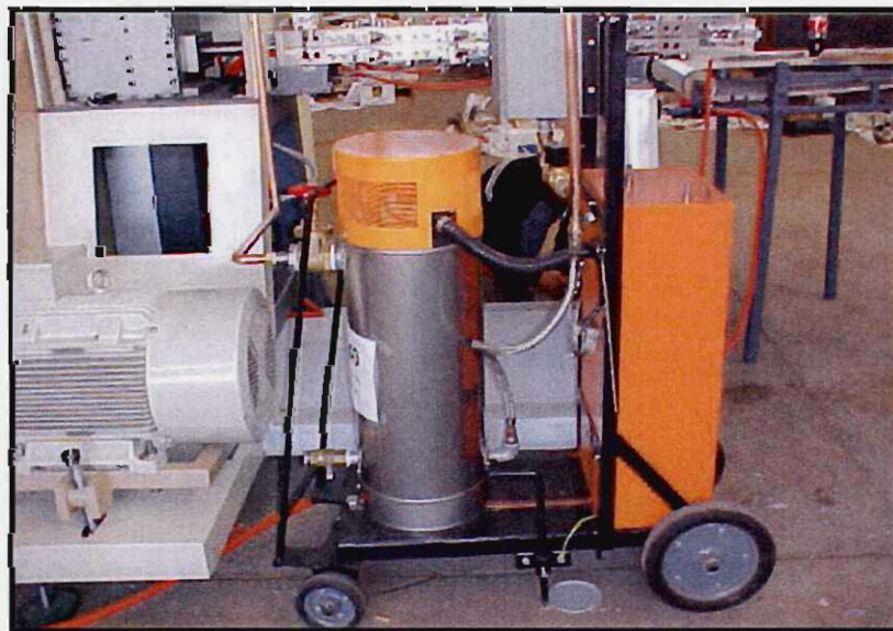
Figure 4.8: Example of a locally manufactured low pressure steam boiler.
