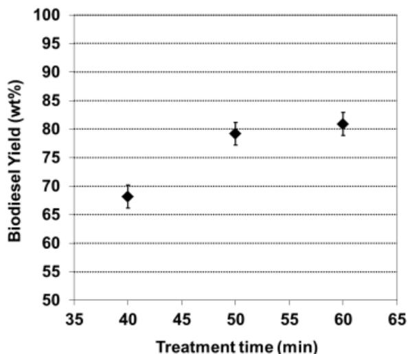
**Figure 5:** Effect of treatment time on the biodiesel yield during ultrasonic assisted biodiesel production
