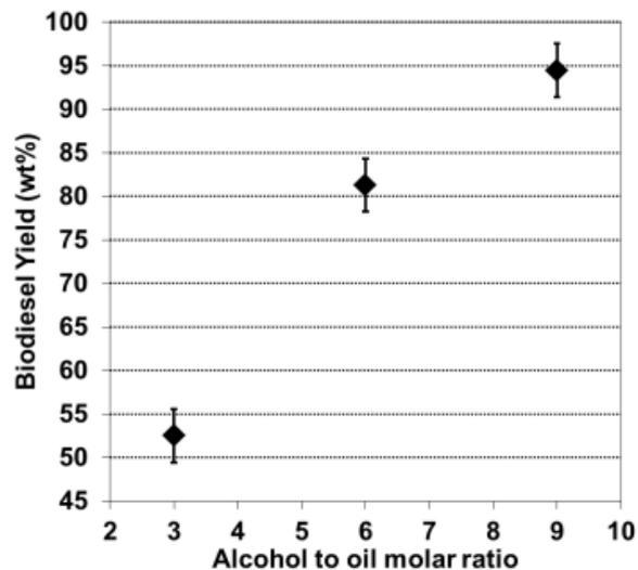
**Figure 2:** Effect of alcohol to oil ratio on biodiesel FAME yield during alkali catalysed transesterification of sunflower oil
