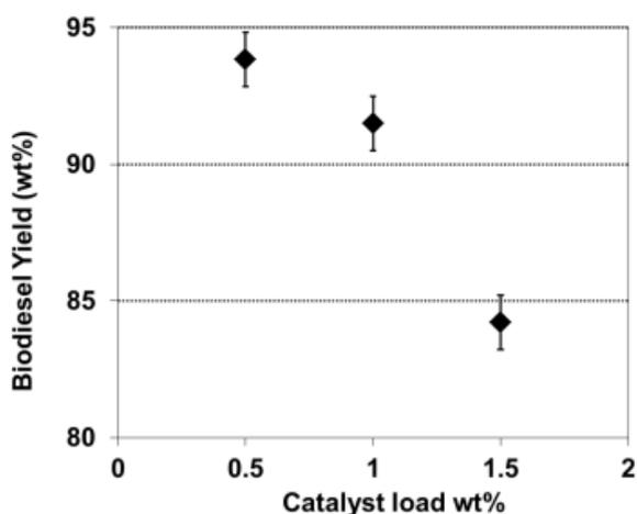
**Figure 4:** Effect of catalyst loading (wt%) on biodiesel layer yield during alkali catalysed transesterification of sunflower oil
