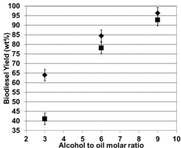
**Figure 1:** Effect of alcohol to oil molar ratio on biodiesel FAME yield during alkali catalysed transesterification of sunflower oil at different ultrasonic frequencies (◆ 35 kHz ■ 130 kHz)
