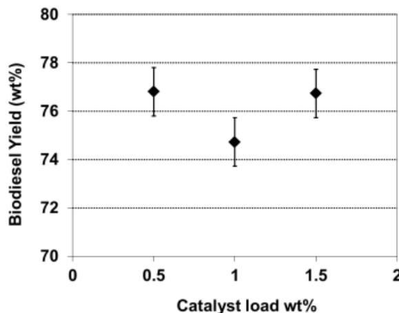
**Figure 3:** Effect of catalyst loading (wt%) on biodiesel yield during alkali catalysed transesterification of sunflower oil
