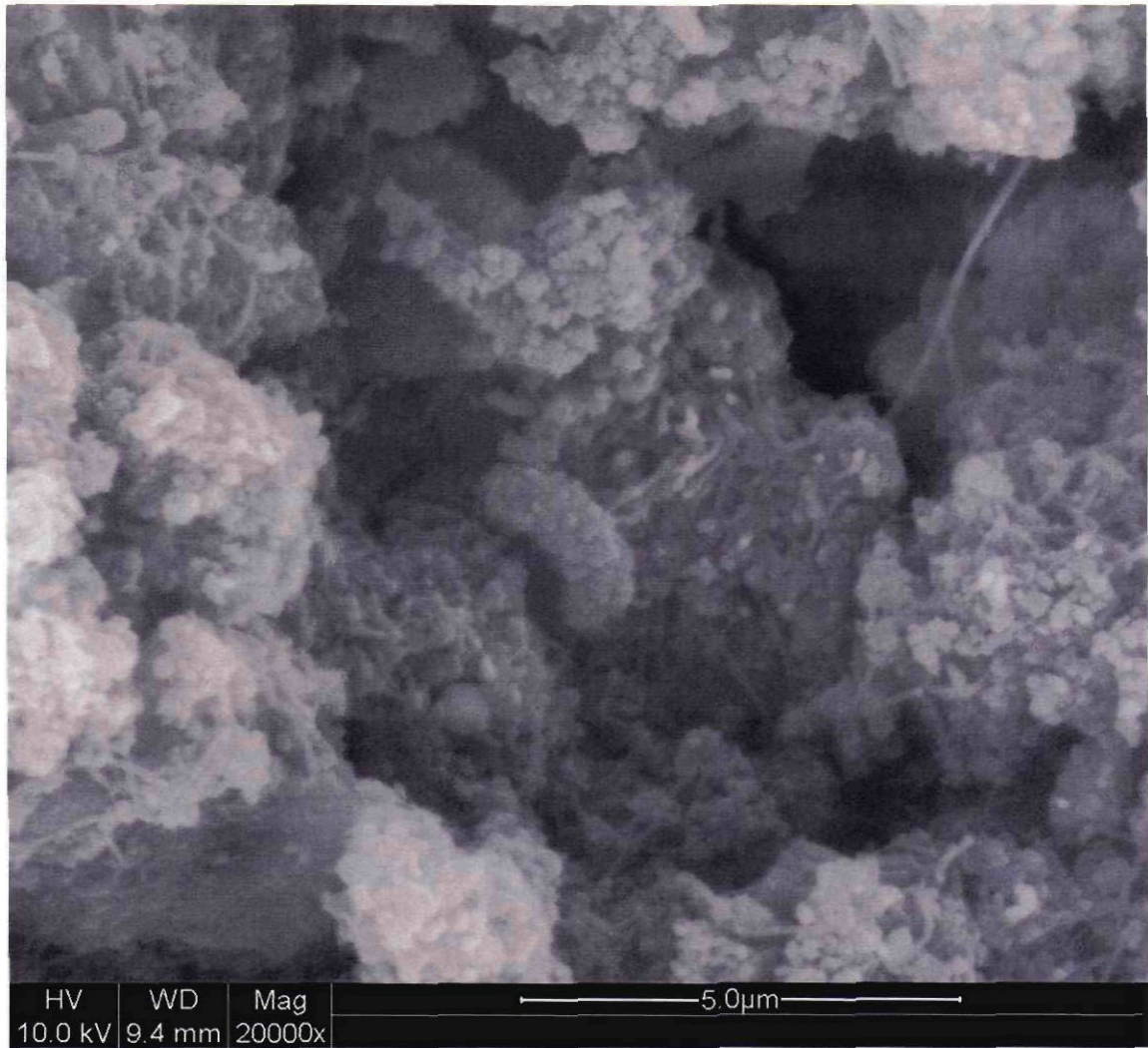
Figure 3.9- Enlargement of the biological activity on the 2 nd phase of the home water filtering system (20 000X magnification).
