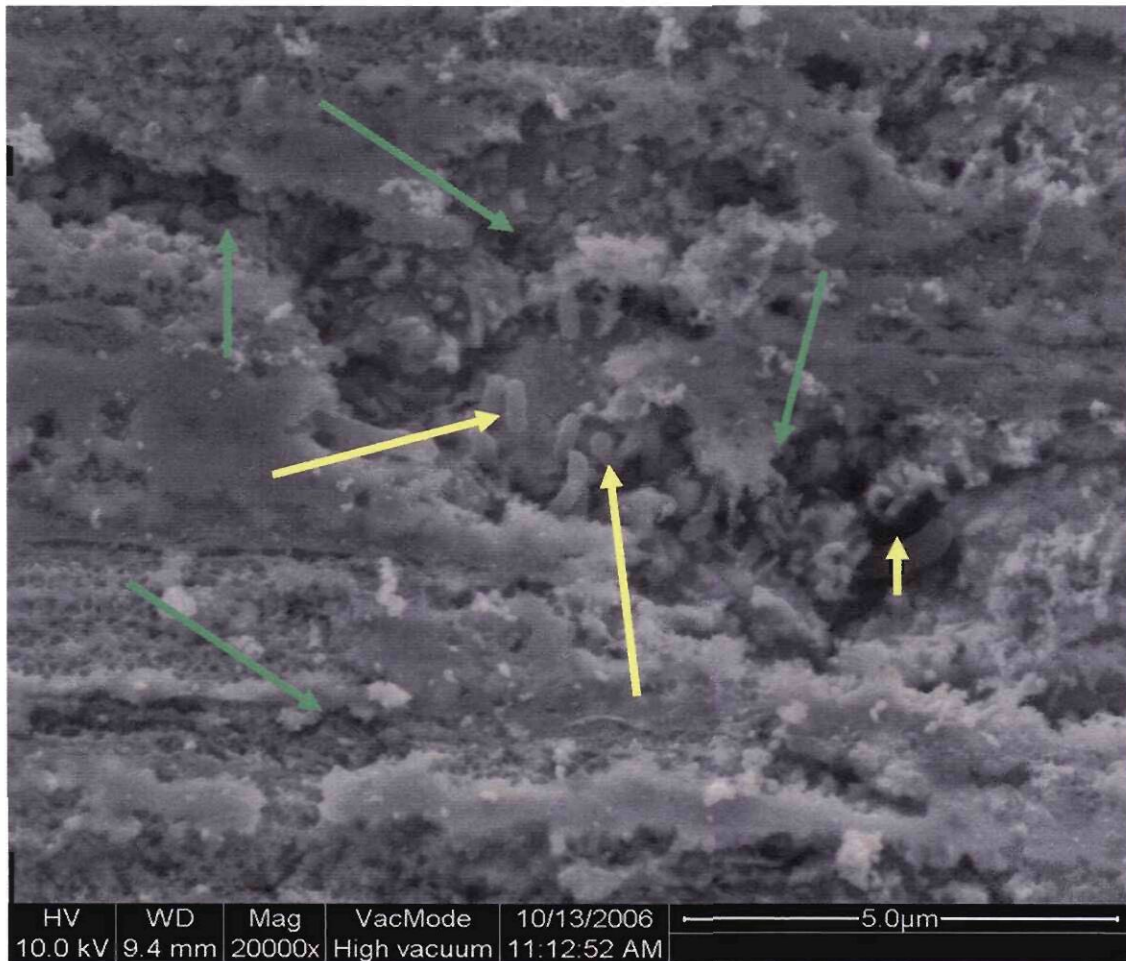
Figure 4.8- A SEM micrograph of a red copper disc after an 8 week period of exposure to drinking water (20 000X magnification).
