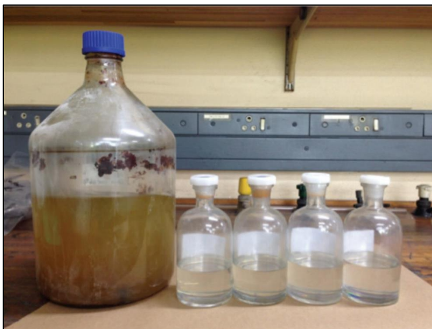
Figure 3-3: Crude \text{TiCl}_4 (left) and four samples of clear \text{TiCl}_4 (right) obtained from distillation (taken from Hockaday and Kale (2016))
