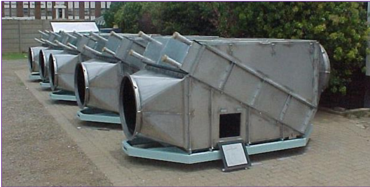
Figure 2-10: 500kW portable Mobile Cooling Unit for use on rail tracks 5
