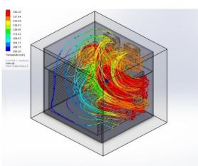
Fig. 7: Simulations with All Fans Active.
