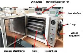
Fig. 13: Complete Integrated System.
