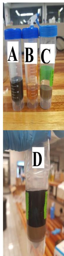
**Figure 6:** Catalyst recovery, A filtrate after microwave pretreatment, B filtrate after NaOH washing, C solid acid catalyst after NaOH washing. D sample before the separation of the solid catalyst and recovered lignin.
