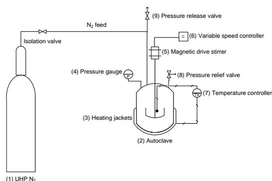
**Figure 1:** Liquefaction reactor setup used in this study
