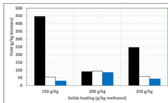
**Figure 5:** Effect of solid loading on biochar (■), bio-oil (□) and FAME (■) yields in the presence of a CaCO<sub>3</sub> catalyst at a temperature of  $330^\circ\text{C}$
