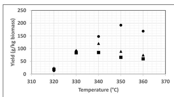
**Figure 3:** Effect of temperature on bio-oil (▲), biochar (●) and FAME (■) yields in the presence of a CaCO<sub>3</sub> catalyst
