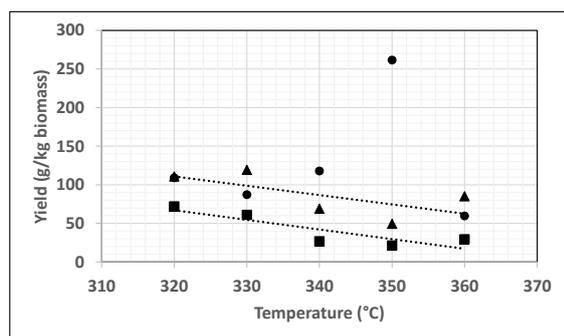
**Figure 2:** Effect of temperature on bio-oil (▲), biochar (●) and FAME (■) yields in the presence of a KOH catalyst
