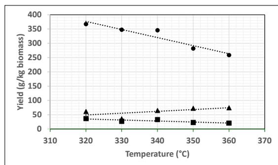
**Figure 4:** Effect of temperature on bio-oil (▲), biochar (●) and FAME (■) yields in the presence of a H<sub>2</sub>SO<sub>4</sub> catalyst
