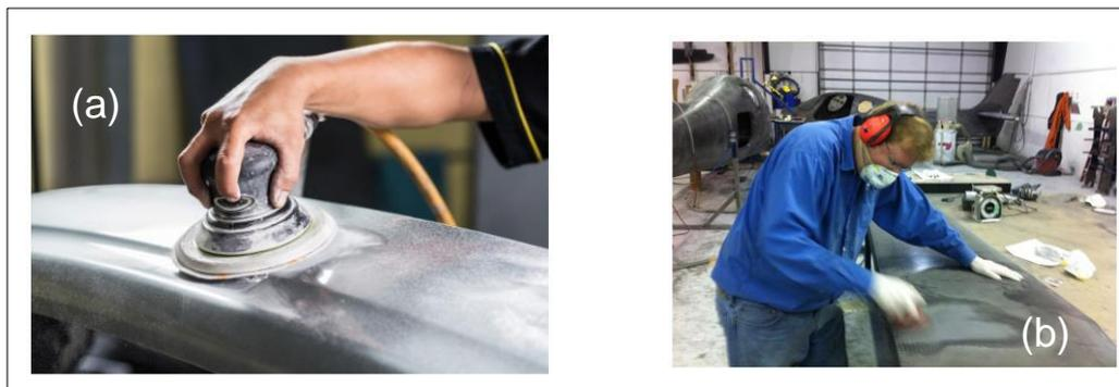
**Figure 2-7: Hand sanding process: (a) orbital sander; (b) sandpaper (Anon., 2019)**
