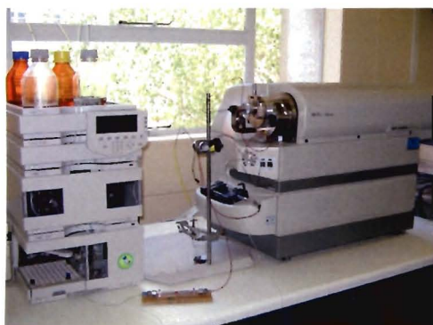
Photo D.11: Agilent 1100 series HPLC coupled to an Applied Biosystems API 2000 triple quadrupole mass spectrometer
