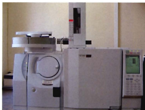
Photo D.12: Shimadzu QP2010 single quadrupole GC/MS with electron ionisation
