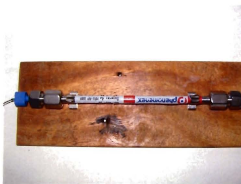
Photo D.10: Synergi C12 column, 150 x 2 mm, 4 \mu m (Phenomenex, Torrance, CA) for LC/MS
