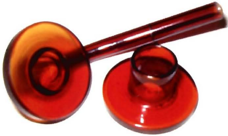
Photo D.1: Vertical Franz diffusion cell with donor and receptor compartments
