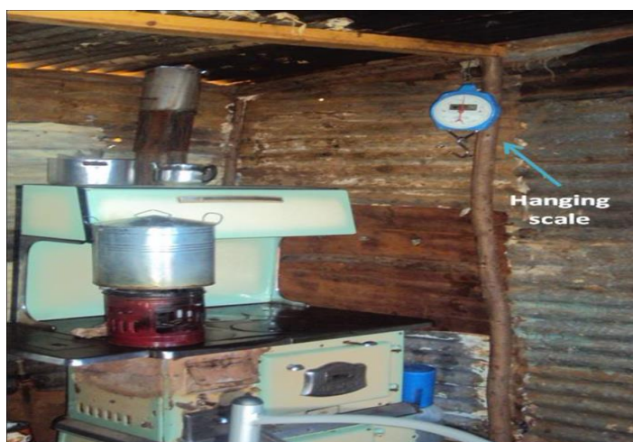
Figure 3.2: A hanging scale set up in a kitchen of one of the 20 study households in Matlwang, where they recorded the mass of the firewood they used (burned) daily
