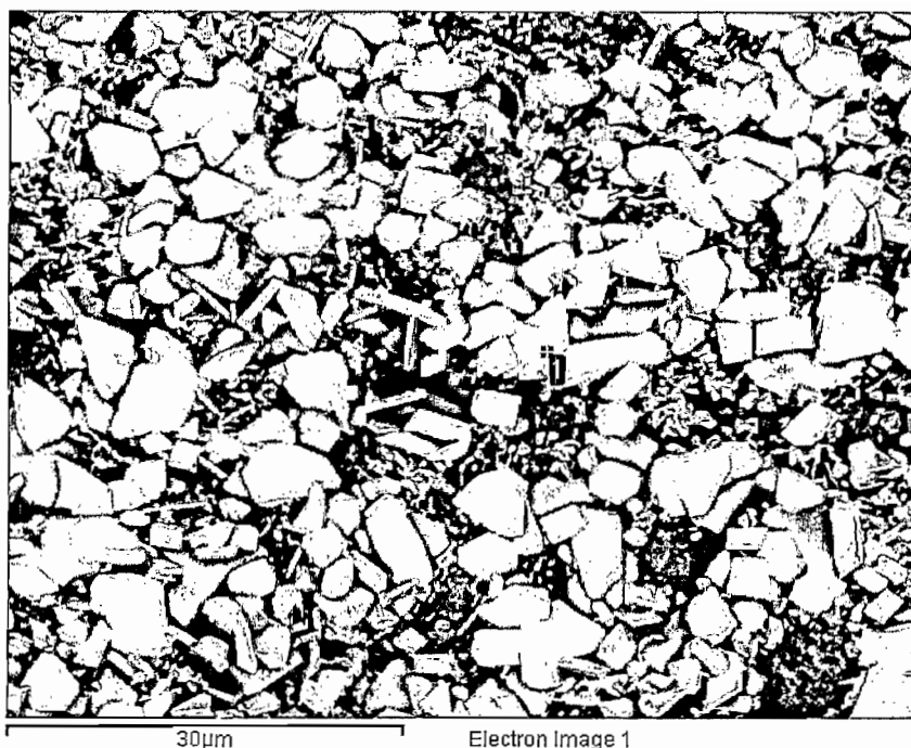
Figure 4.5 Micrograph of crystals on lid of crucible, in which a chromite/carbon/attapulgite mixture containing 5% NaCl was treated at 900°C in a partially reducing atmosphere
