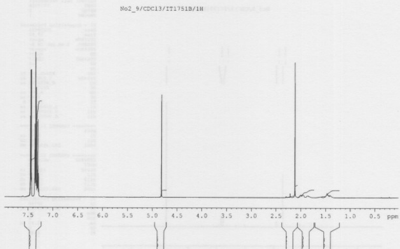
Spektrum 4.28 ^1\text{H} KMR van die reaksie van BDD (in PhCl) en \text{PCy}_3 (in PhCl) by 80 °C na 2h (Ru: \text{PCy}_3 :BDD = 1:2.5:10).
