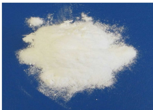
Figure 5.20 Photograph of the pure, white high-grade \text{CaCO}_3 product produced in the indirect CaS carbonation process
