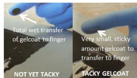
**Figure 5-8: Tacky Gelcoat test**
