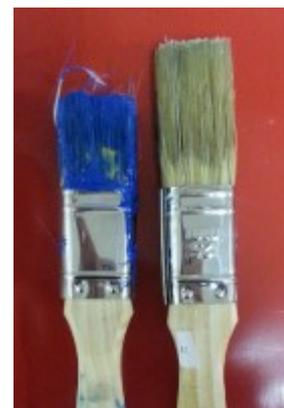
**Figure 5-7: Brush cut shorter for gelcoat**
