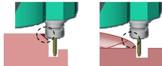
*Figure 5-3: Provision for tool shanks versus depths of cuts.*
