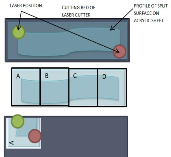
**Figure 5-5: Improved cutting method for laser cutting of plug split surfaces.**
