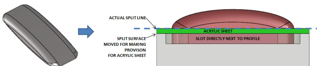
**Figure 5-1: Surface finish provisions of the plug.**
