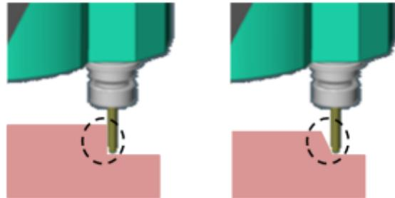
*Figure 5-2: Draft angles on parts preventing scuff marks on side walls of plug*
