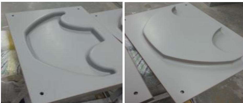
*Figure 6-2: Plugs after sanding to P3000 grit and polishing to a Class A finish*
