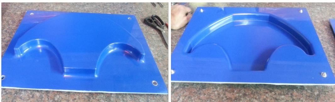
*Figure 6-5: Finished top and bottom moulds*
