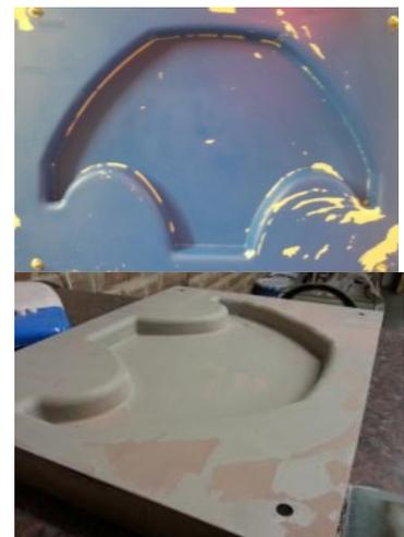
*Figure 6-4: Mould and plug surfaces directly after demoulding.*
