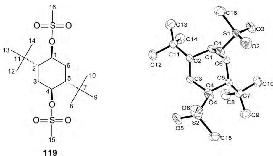
**Figure 4.7** Bis(methanesulphonate) ester (**119**) (XRD hydrogen atoms are omitted for clarity).
