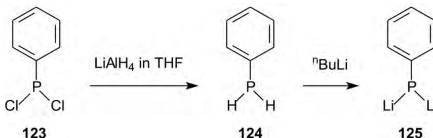
**Scheme 4.9** The synthesis of dilithium phenylphosphine **125**.
