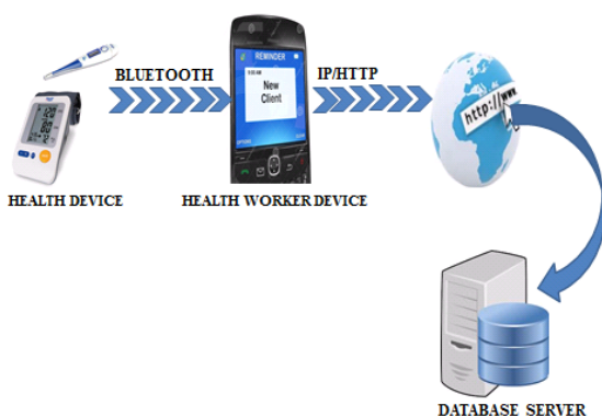
Figure 1: Mobile health system communication
