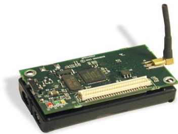
Figure 1: Figure taken from [2], XM2110 Crossbow Iris Mote with Standard Antenna.
