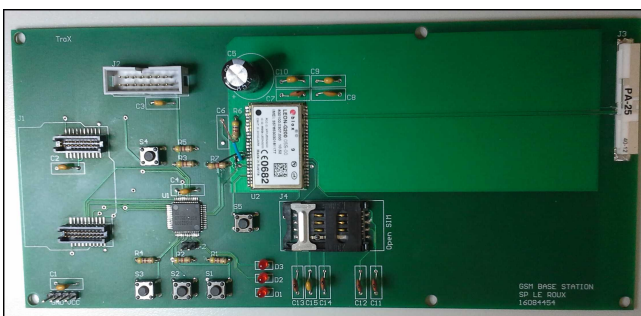
Fig. 6. Assembled Base Station
