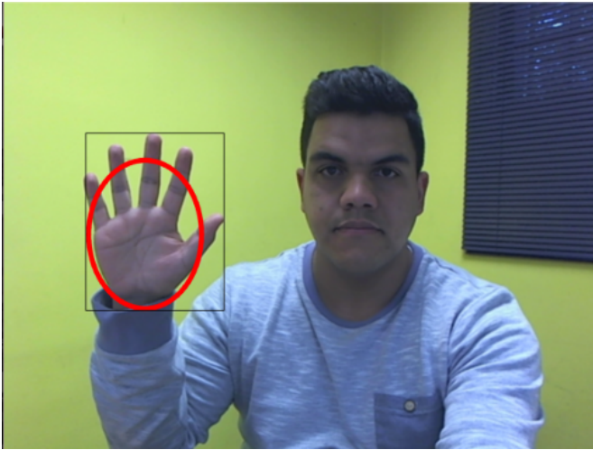
Fig. 4. An ellipse around the tracked hand using the CAMShift tracking algorithm.
