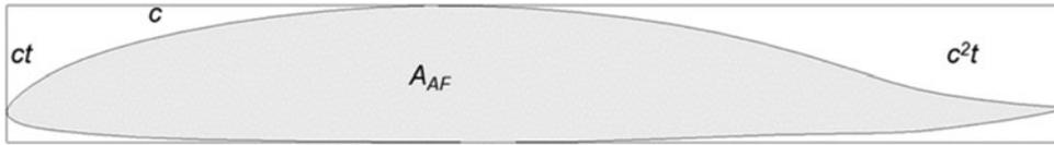
Figure 6. An aerofoil comparable to the DU97 of thickness  $t = 12.7\%$  has an area fraction  $f_{AF} = 68.4\%$ .
