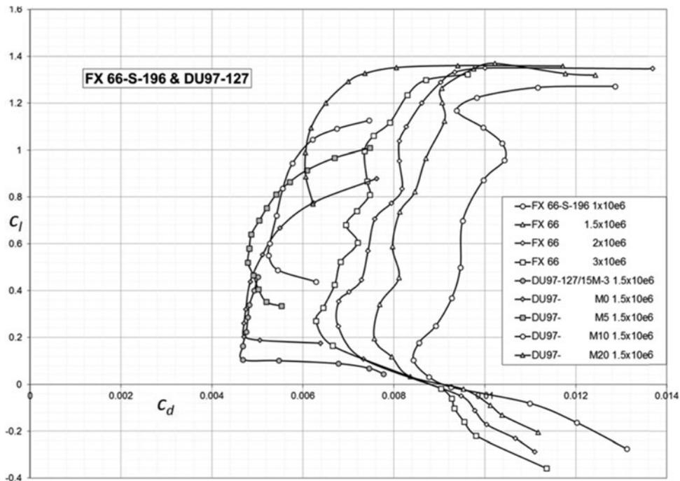
Figure 3. Experimental data of the Wortmann FX 66 aerofoil<sup>(22)</sup> at different Reynolds numbers and the Delft DU97 aerofoil<sup>(19)</sup> at different flap settings. For each polar curve, only the laminar ‘drag bucket’ is shown.
