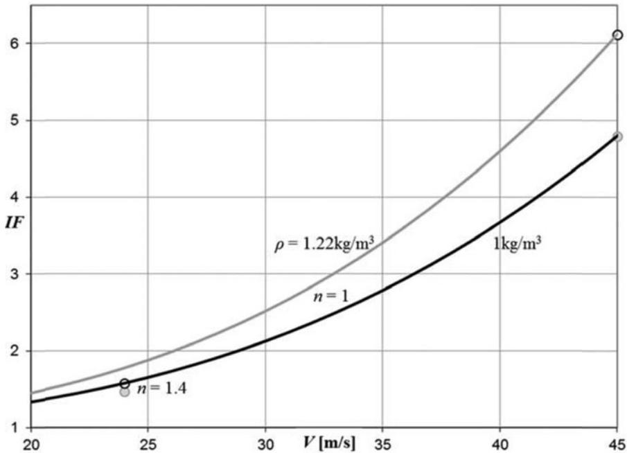
Figure 7. Inflation factor ( $IF$ ) as a function of the design flight speed  $V$  for different air densities  $\rho$  and load factors  $n$  (based on the aerofoil parameters offered in the previous figures).
