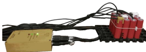
Figure 4. Battery pack setup with sensors and DAQ
