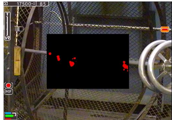
Figure 11. Visualization with one pipe on at +100 kV
