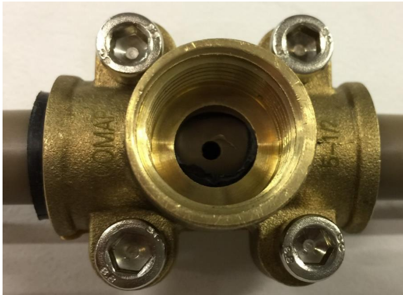
Figure 2: Photo of the 2mm leak applied to the Experimental Network
