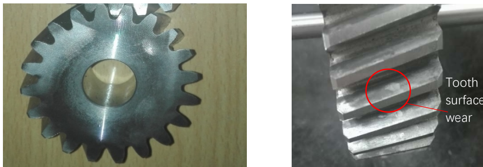
Figure 5. Normal helical gear and faulty helical gear
