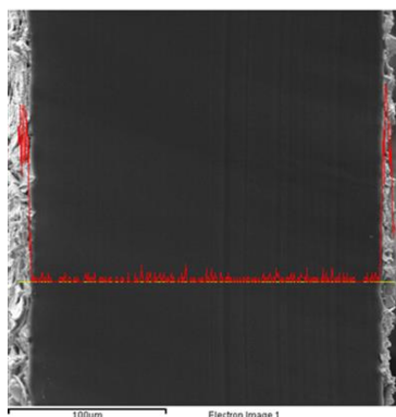
Figure 5.2: Typical Pt morphology by SEM of the membrane cross-section produced by HySA
