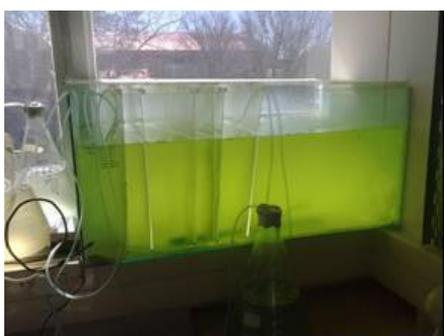
**Figure 7:** Hartbeespoort Dam microalgae growth in 135-litre glass tank bioreactor after two weeks of cultivation
