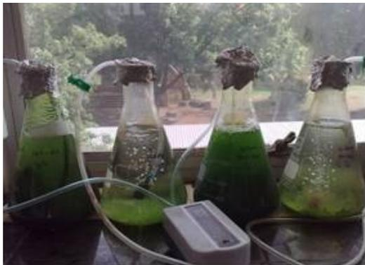
**Figure 2:** Hartbeespoort Dam microalgae growth in 1-litre Erlenmeyer bioreactors after three weeks of cultivation
