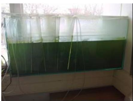
**Figure 8:** Hartbeespoort Dam microalgae growth in 135-litre glass tank bioreactor after six weeks of cultivation
