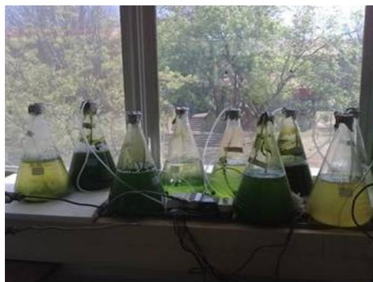
**Figure 5:** Hartbeespoort Dam microalgae growth in 5-litre Erlenmeyer bioreactors after six weeks of cultivation
