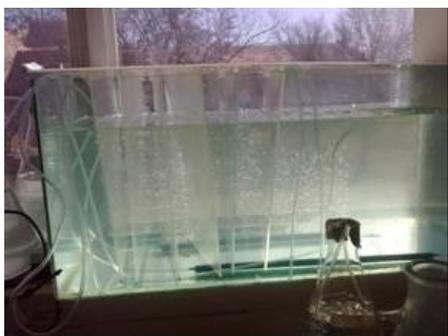
**Figure 6:** Cultivation of Hartbeespoort Dam microalgae in glass tank bioreactor with growth plates
