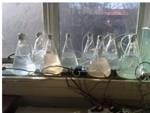
**Figure 3:** Hartbeespoort Dam microalgae inoculated in 4-L Erlenmeyer bioreactor flasks
