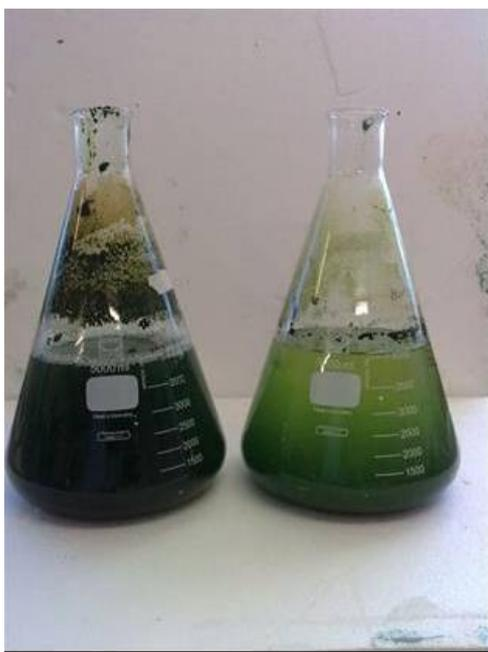
**Figure 4:** Gravitation settling comparison between well-mixed bioreactor (left) and bioreactor that was allowed to settle for 24 hours
