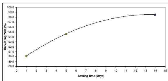
**Figure 6:** Harvesting yield of cultivated micro-algal biomass sourced from the Hartbeespoort Dam versus gravity settling time in the bottom 25% of three Erlenmeyer bioreactors: (○) bioreactor 1; (□) bioreactor 2; (△) bioreactor 3; The solid line does not constitute a fit, but just a visual guide.
