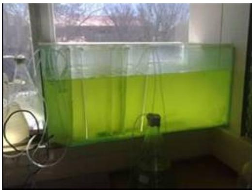
**Figure 1:** Cultivation of microalgae in 135-litre glass tank bioreactor with Perspex growth plates
