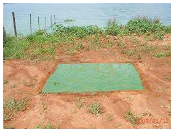
Figure 4: 4 m 2 patch of cleared soil containing a layer of harvested wet Hartbeespoort Dam micro-algal biomass
