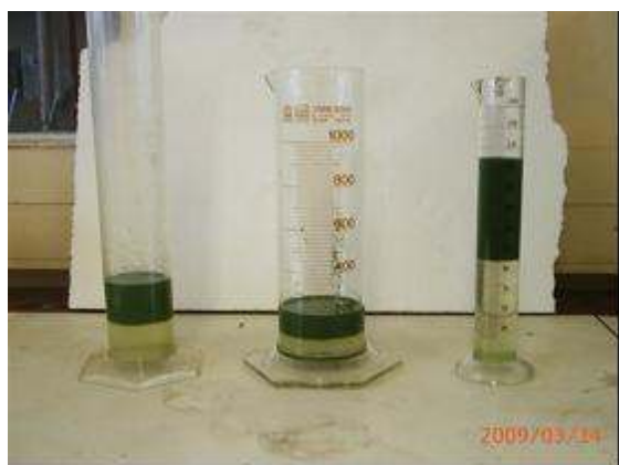
Figure 2: Hartbeespoort Dam microalgae separating to the top of the measuring cylinders after 3.5 hours at a concentration of 3% TSS
