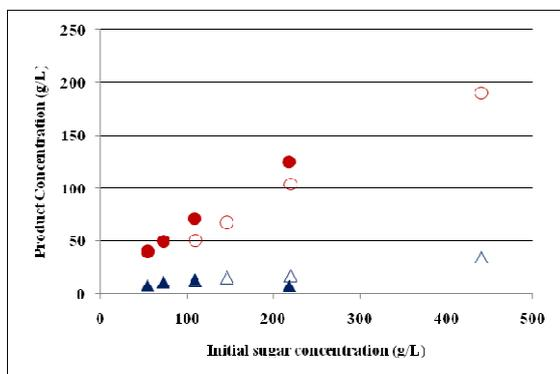
**Figure 2:** Effect of initial sugar concentration on ethanol and glycerol concentration in the fermentation broth after 12 hours of fermentation
