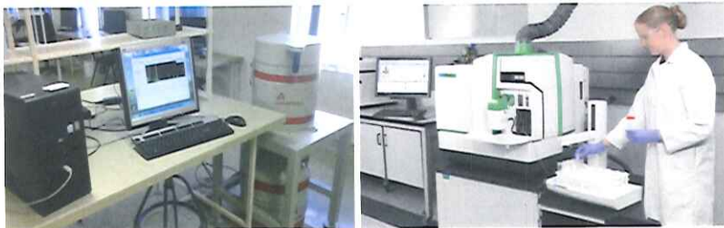
High Purity Germanium Detector (HPGe) (LHS) and NexION 2000Q ICP-MS (Perkin Elmer) (RHS)
