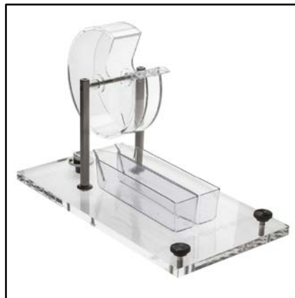
Figure 2.7: Folsom plankton splitter with collecting containers.
