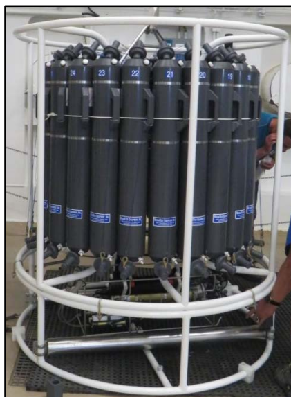
Figure 2.8: Conductivity, Temperature, and Depth (CTD) sampler with 24 fitted 12 L collecting bottles.
