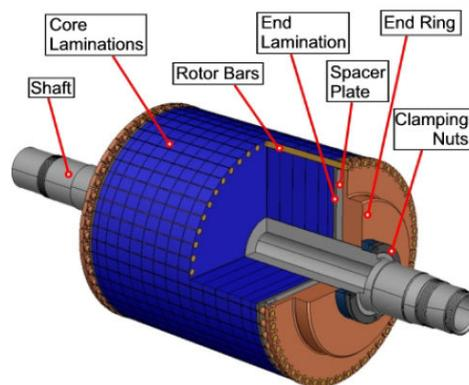
Figure 2-2: M.T. Caprio, V.L. John and J.D. Herbst, rotor configuration [9]
