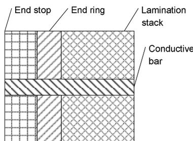
**Figure 2-18: L.M. Mhango's end stop design feature [4]**
