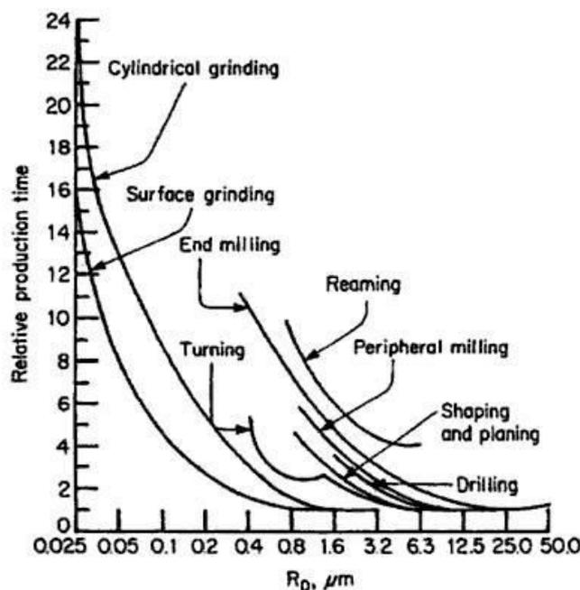
Figure 2-21: Comparing time required to obtain a specific surface roughness using different manufacturing processes [46]
