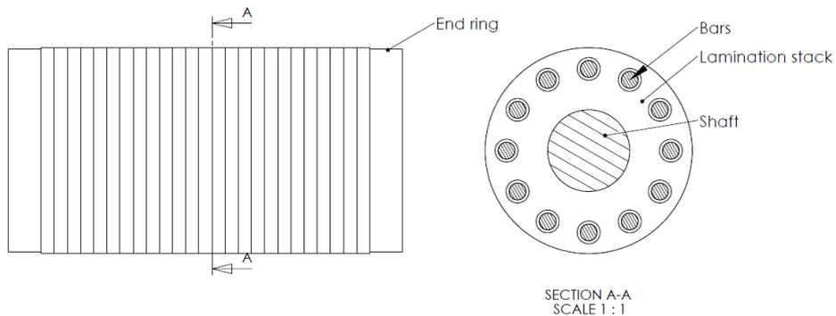
Figure 2-6: Laminated cage rotor illustration
