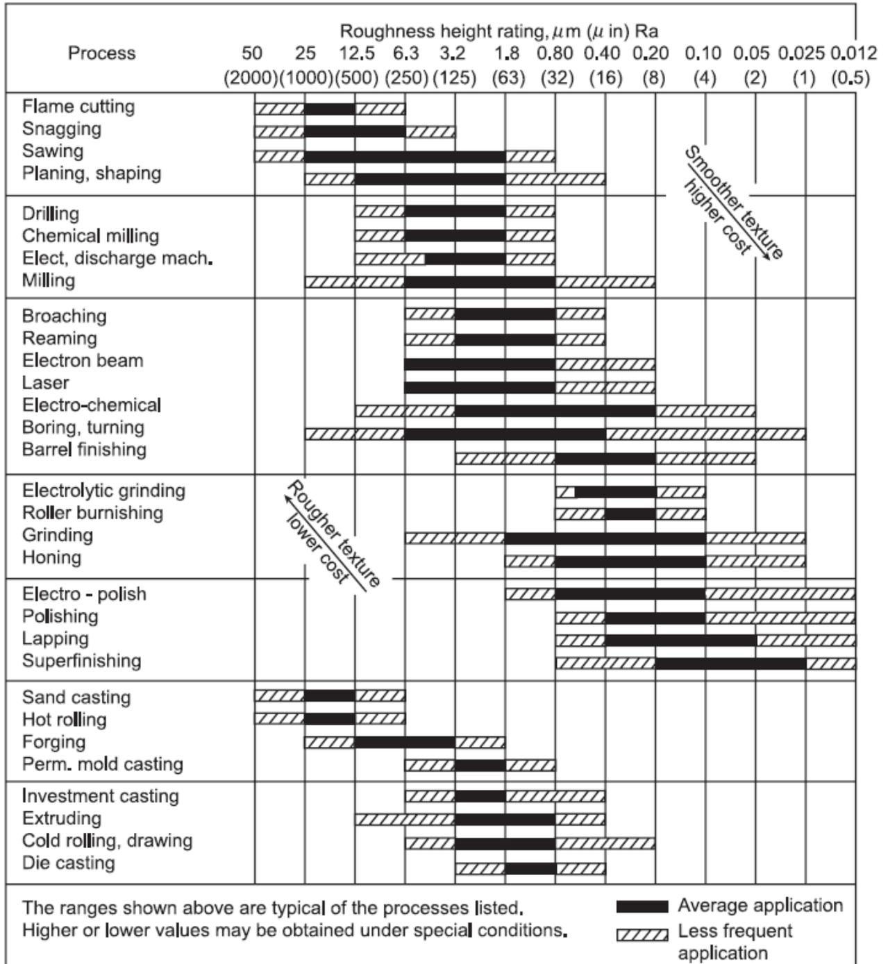
Figure 2-22: Typical surface roughness for specific manufacturing processes [47]
