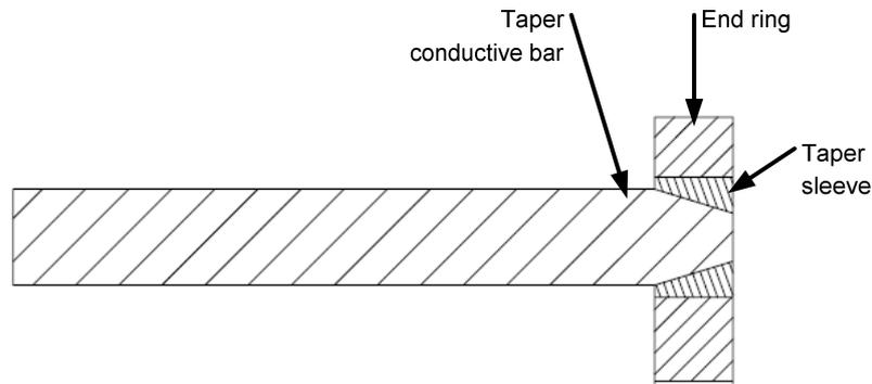
**Figure 2-12: Section view of taper interference fit bar/end ring connection**
