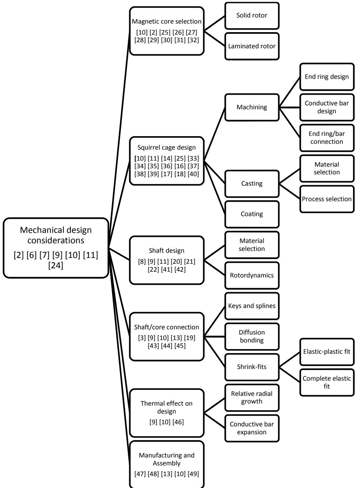
Figure 2-1: Mechanical design considerations detail breakdown
