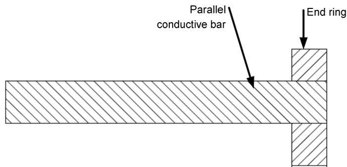
**Figure 2-13: Section view of parallel interference fit bar/end ring connection**
