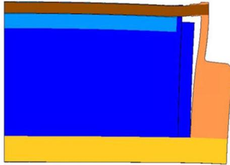
Figure 2-8: Exaggerated deformation due to temperature [9]
