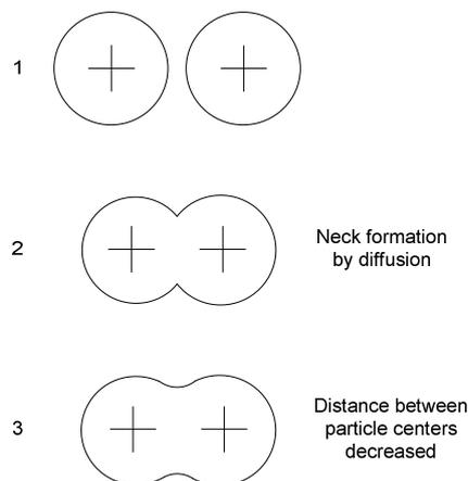
**Figure 2-15: Schematic illustration of the solid-state diffusion bonding mechanism [13]**
