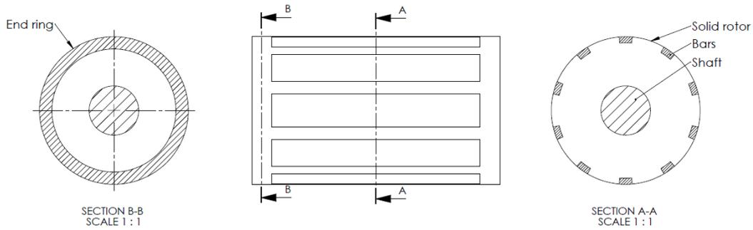
Figure 2-5: Solid cage rotor illustration
