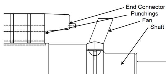
Figure 2-11 Traditional IM rotor construction [15]
