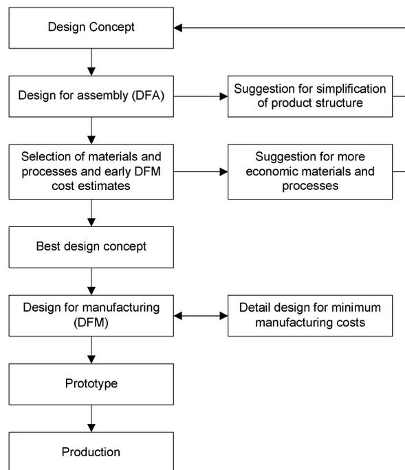
Figure 2-20: Typical DFMA procedure used by DFMA software [23]
