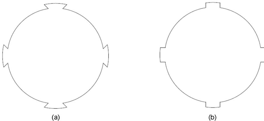
**Figure 2-14: (a) Illustrates a dove-tail and (b) a square spline shaft**
