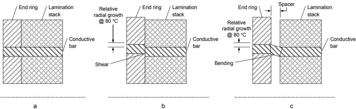
Figure 2-16: Shear and bending in the rotor bars due to elevated operating temperatures
