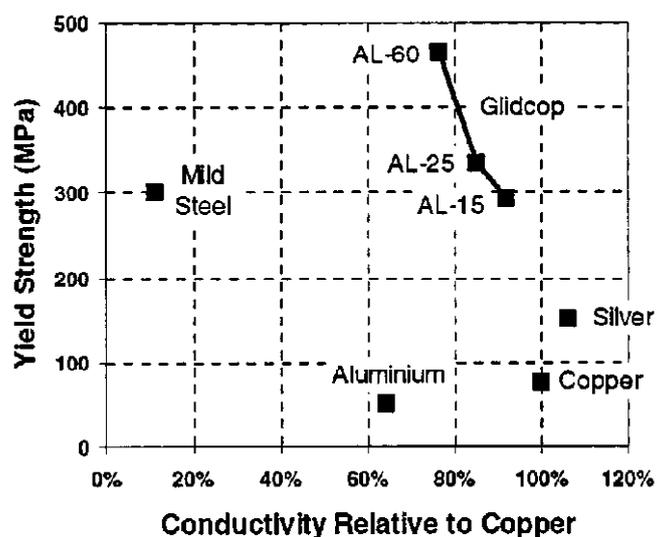
Figure 2-10: Rotor cage material trade off between conductivity and strength [7]
