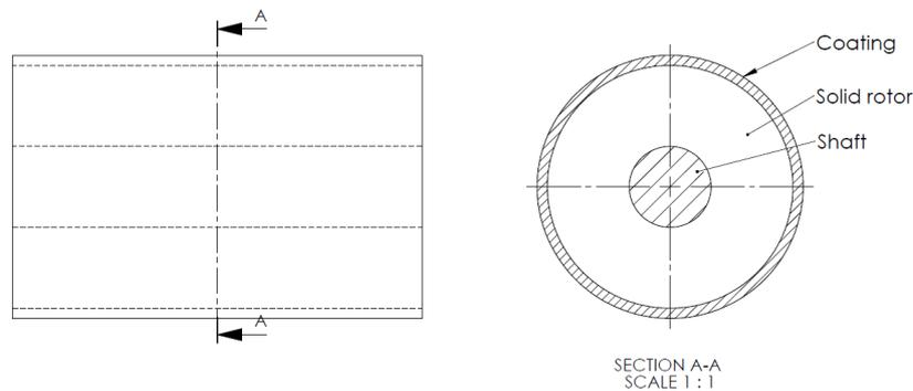
**Figure 2-4: Solid coated rotor illustration**
