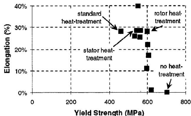
Figure 2-3: Rotor lamination material's tradeoff between strength and ductility [7]
