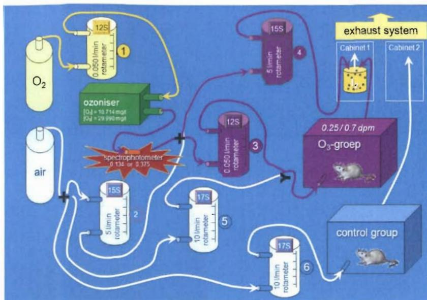
**Figure 3:** Schematic representation of an ozone inhalation setup for rats.
